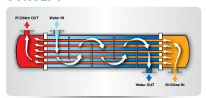
The single pass shell and tube evaporator makes it possible to achieve excellent thermodynamic efficiency values thanks to the complete countercurrent in the heat exchange.
