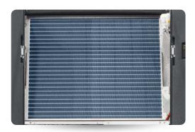
All models in the **JREF DX** range feature heat exchange coils with **hydrophilic coating**. This special coating - together with an adequate adjustment of air through-flow speeds - helps condensate collection during the dehumidification process, avoiding dripping on the inside and outside of the unit.
